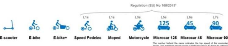
The number behand the name indicates the top speed of the exemplary model. The maximum design speed is lended by law to 40 km/h for category (b), to 90 km/h for category L7 or and is not lended for category L5e.
